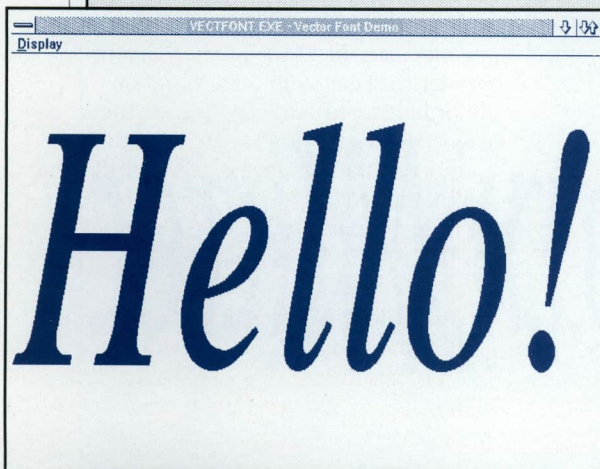
Figure 4 A vector font stretched to fill the client window, displayed by selecting Stretched Font from the VECTFONT menu.
