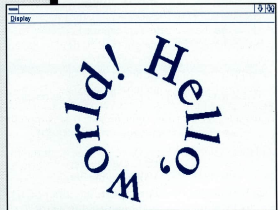
Figure 7 Character string displayed around the perimeter of a circle, displayed by selecting Rotated Font from the VECTFONT menu.
