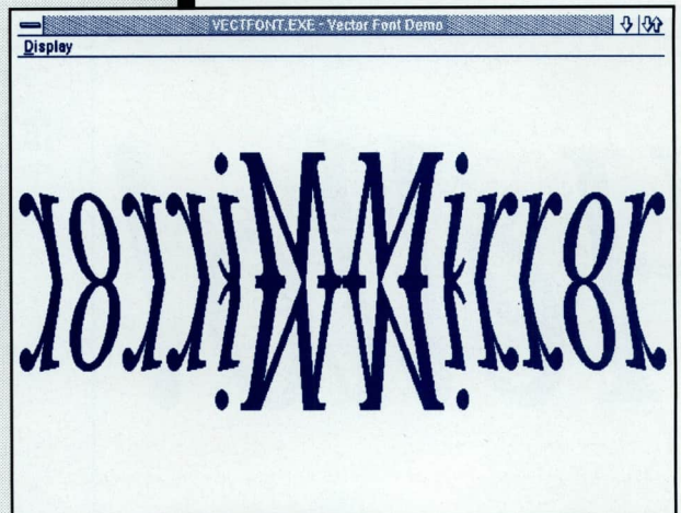
Figure 5 Vector font with positive and negative character box values, displayed by selecting Mirrored Font from the VECTFONT menu.
